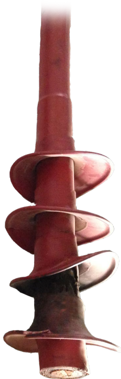
Cable head failure due to Partial Discharge
